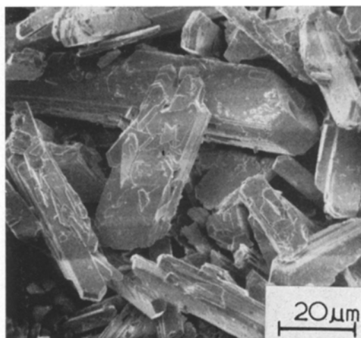
Figure 3 Lath-like morphology of ammonium paratungstate (sample 1).
